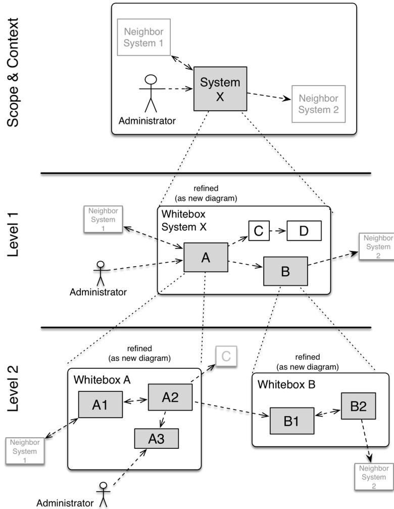
**Level 1** is the white box description of the overall system together with black box descriptions of all contained building blocks.
